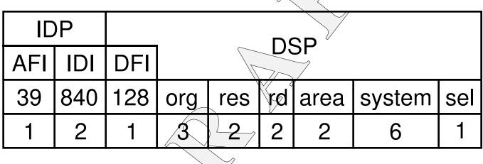
Figure 1 — Structure of the DSP
